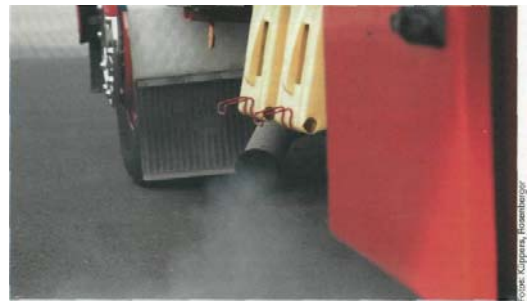
Various retrofit models filter practically all particulate matter from exhaust gases
