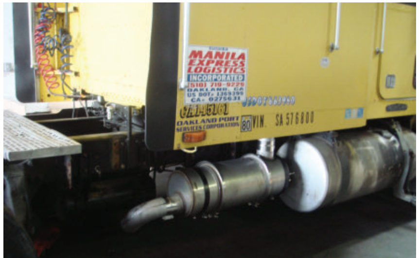
Retrofits on trucks such as this 1994 Freightliner with a Detroit Diesel Series 60 took an average of six to eight hours, depending on which Purifilter system was used.
